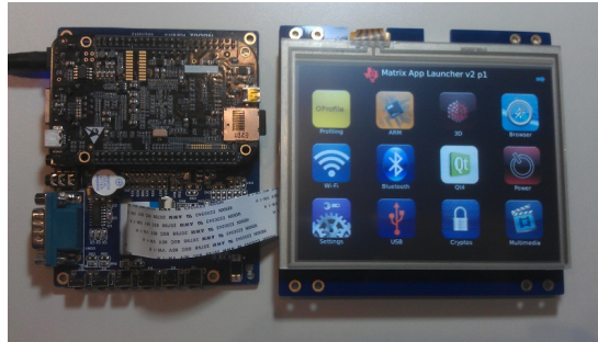
Figure 2: BeagleBone Black running Android OS during the performance evaluation.
