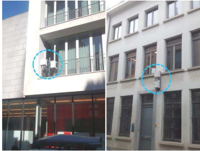
Fig. 2. Example of gateway deployment in the city of Antwerp available for remotely wireless experimentation.
